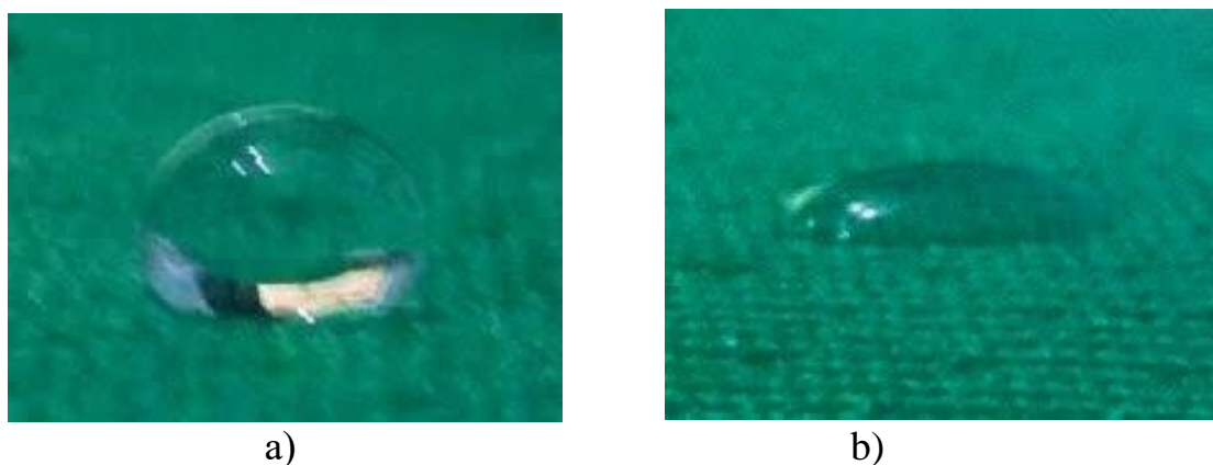
Figure. 2. The effect of treatment with the drug 102-SG on the change of the edge angle wetting of PA knitwear samples ( \times 10 ):
